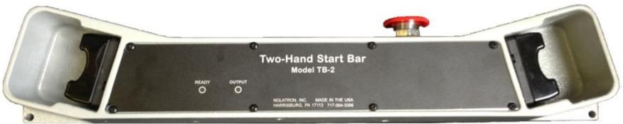
The Start Bar is an ergonomic starting system. The internal anti-tiedown control monitors both start sensors for concurrent operation. The output utilizes redundant positive guided relays which are monitored to ensure proper operation.
