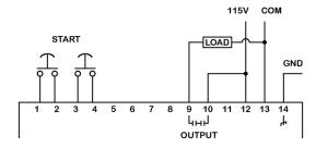
**TIMED OUTPUT:** Both start switches must be pressed within .5 seconds\* to energize the load. The load will remain energized until the time cycle is completed or one or both start switches are released.
