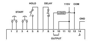
MAINTAINED and DELAYED TIMED OUTPUT: Both start switches must be pressed within .5 seconds\* to energize the load. When the Hold switch is closed, the load will remain energized for the remainder of the time cycle, even if the start switches are released. The time cycle will not begin until the Delay switch opens.
