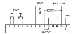
**DELAYED TIMED OUTPUT:** Both start switches must be pressed within .5 seconds\* to energize the load. The load will remain energized until the time cycle is completed or one or both start switches are released. The time cycle will not begin until the Delay switch is opened.
