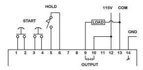
**MAINTAINED TIMED OUTPUT:** Both start switches must be pressed within .5 seconds\* to energize the load. When the Hold switch is closed, the load will remain energized for the remainder of the time cycle, even if the start switches are released.
