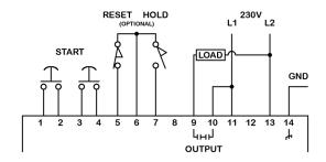
**OPERATION:** As each start switch is closed, it will be delayed for .075 seconds\* before an internal relay is energized. If both start switches are closed within a time of .5 seconds\*\*, the output contact will close and the load will energize. The output contact will remain closed until one or both start switches are opened. Both switches must be released before another cycle is initiated.
