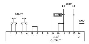
The 4480-TC includes the optional normally closed contact feature between pins 8 and 10. The normally closed contact on pin 8 is not monitored, and should not be used to drive a load that needs "control reliable" protection.
