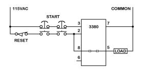
**MAINTAINED OUTPUT:** Adding the optional Hold switch will allow the load to remain energized after the start switches are released. *The Hold switch must not be closed until the pinch point is passed.* The Hold switch should stay closed for the rest of the machine cycle. If the Hold switch is opened after one or both switches are released, the load will de-energize.
