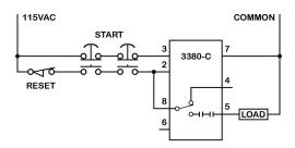
**MAINTAINED OUTPUT:** Adding the optional Hold switch will allow the load to remain energized after the start switches are released. *The Hold switch must not be closed until the pinch point is passed.* The Hold switch should stay closed for the rest of the machine cycle. If the Hold switch is opened after one or both switches are released, the load will de-energize.
