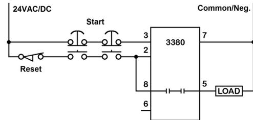
**MAINTAINED OUTPUT:** Adding the optional Hold switch will allow the load to remain energized after the start switches are released. *The Hold switch must not be closed until the pinch point is passed.* The Hold switch should stay closed for the rest of the machine cycle. If the Hold switch is opened after one or both switches are released, the load will de-energize.
