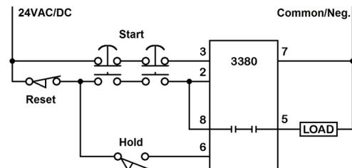
**Note: The Reset and Hold switches shown in the above wiring diagrams are optional and are not required for all applications**
