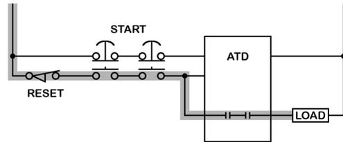
**LOAD TRANSIENT DAMAGE:** If the load is a solenoid, a motor, a relay coil or a transformer, it will have inductive properties. When a relay contact breaks the current to an inductor, a high voltage will result across the contact. This high voltage may damage the contacts when they begin to separate. Good transient suppression (placed across the load) can greatly reduce this damaging high voltage and increase operating life.
