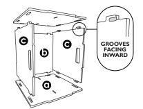
Lay side **(a)** on the ground with the slots facing up. Insert bottom **(b)** and ends **(c)**, placing other **(d)** on top.
