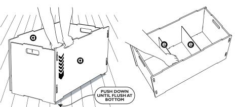
Place crate on hard floor, then press down each corner in turn to tighten.
