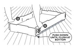
Place tray on hard floor, then press down each corner in turn to tighten.
