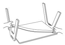
Rotate and insert ends of Brace **(B)** into slots on underside of Legs **(A)**.
