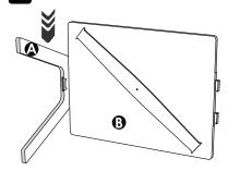
Rotate assembly 180°. Repeat step 1-2 with the second Leg (A).
