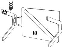
Carefully bend up both ends of the Brace (3).
