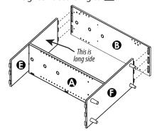
Turn unit onto Side **(B)** as shown. Insert Back **(D)** then Left Side **(E)**. Tighten according to **(A)**.
