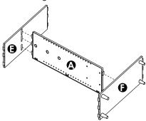
Pop Right Side (B) over tabs of Top Shelf (B) and Bottom Shelf (F). Then tighten according to (A).
