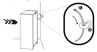
Thread the end of the Zip Tie up through the D-Ring as shown. Push the unit closer to the wall if needed.
