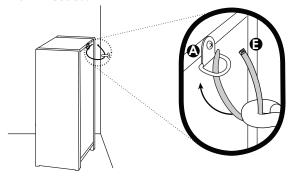
Thread the end of the Zip Tie through the head. Slowly pull tight while pushing the unit closer to the wall.
