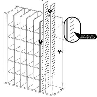
With another adult holding the Assembly Jigs (steady, slide all Slot Dividers (e) into their slots on Middle Shelf (f), as shown. Assembly Jigs will help hold the Slot Dividers in place.
