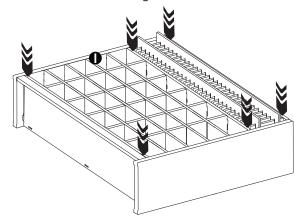
Carefully wiggle Assembly Jigs **()** to remove. With another adult, carefully tilt unit up onto feet.
