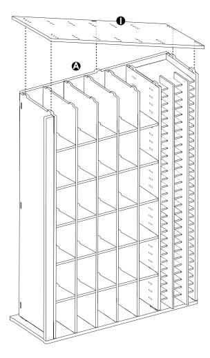
Lock tabs on Left Side **1** and check that all other tabs are locked and edges are flush. Refer to **4**.
