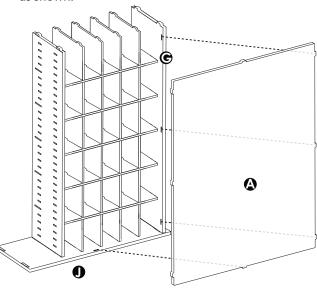
With another adult holding the assembly steady, place (1-2) Assembly Jigs next to Middle Shelf on the front edge of the unit with slots facing in towards the Back .
