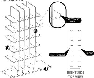
Place tabs for Bottom (and Middle Shelf (in slots of Right Side (i), as shown. Large slots on Middle Shelf should be towards front of unit. Insert tabs of Dividers into slots on Bottom and Middle Shelf, and tighten Bottom (in slightly).
