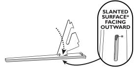
Remove Bracket from Leg **3**, and slide end of Leg into slot on Table Top **3**.
