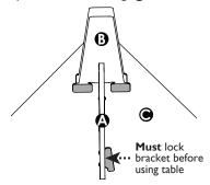
Install Rib **①** by inserting first two tabs into corresponding slots on Table Top **③** . Note that tabs will not slide in completely until next step.
