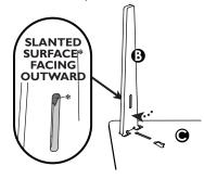
Insert Bracket **(A)** tip into slot on Leg **(B)**, and rotate down bottom corner.
