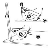
Bend tip **X** of Bracket **(A)** over and down into slot.
