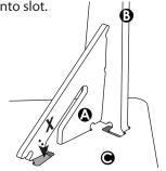
Push Bracket **(A)** in to lock in place. Repeat steps 1-5 for each Leg **(B)**.
