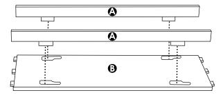
Turning the part upright, push down on Toes **(A)** until the ends are flush with the ends of Bottom **(B)**. Repeat with second Toe.
