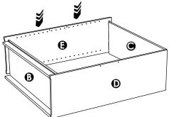
Carefully tilt unit up on Bottom 3. Install Back by aligning with pilot holes on Sides. Thread Screw through pilot holes with provided Allen Wrench 1.
