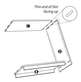
Press or hammer down Left Side **①** to tighten until it makes contact with the ground. It will be flush with the underside of Top **②** and Bottom **③**. Parts will be snug. Remove excess glue from joints with a damp cloth.
