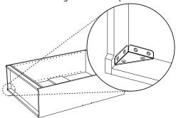
3 Using a drill or power screwdriver, install 2 screws into the holes on the triangular face. Make the screws as straight as possible.
