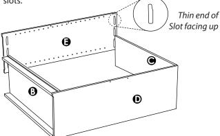
To tighten, press or hammer down Right Side (a) until it makes contact with the floor. Parts will be snug. Remove excess glue from joints with a damp cloth.
