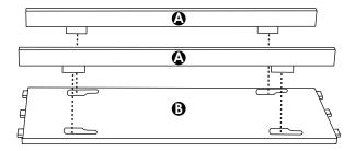
Turning the part upright, push down on Toes **(A)** until the ends are flush with the ends of Bottom Shelf **(B)**. Repeat with second toe.
