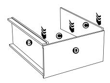
One adult holds steady Side **①**, Shelves **②** and Bottom **③**. Apply glue to the tabs on **③** and **⑤** and the slots of the other Side **①**. Pop tabs into corresponding slots.
