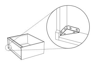
Using a drill or power screwdriver, install 2 screws into the holes on the triangular face. There are no pre-drilled holes in the wood, so try to make the screws as straight as possible.
