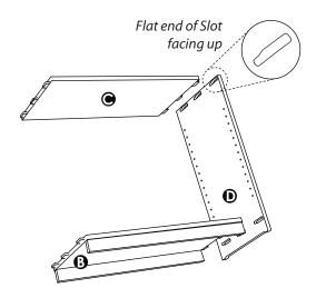
Press or hammer down Shelves and Bottom to tighten until they make contact with the ground. They will be flush with the underside of Side Parts will be snug.
