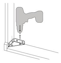
Install 2 more screws into the holes on one of the small sides of the bracket, then the other.
