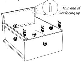
To tighten, press or hammer down the second Side **1** until it makes contact with the floor. Parts will be snug. Remove excess glue from joints with a damp cloth.
