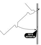
To remove from slotboard, pull up firmly to pop out bottom tab.
