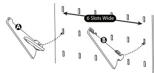
Press the bracket tips inward to tighten braces completely.
