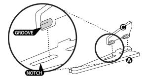
Tighten slightly by pushing down on the large end of the Brace **(G)**. Will finish tightening in Step 4.
