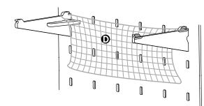
Pull other corners of Net **①** over front tabs of Brackets, then straighten Brackets as needed.
