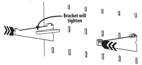
Put corners of Net **①** over back tabs of Brackets.
