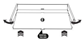
Put slots on Front **(A)** onto tab on Left Side **(3)**& dovetail on Bottom **(5)**.
