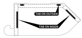
Carefully press the tabs of the three panels into the slots, orienting them per .
