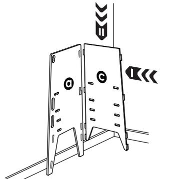
**1** Push tabs on Back (c) into slots on Left Side (c). Push down on Back (c) to lock into place.
