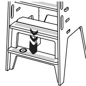
**5** Step on Ladder (e) to lock into place.
