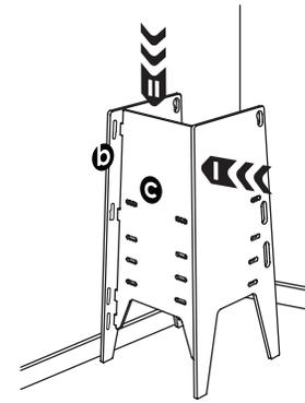
**2** Turn parts around, then push tabs on Back (c) into slots on Right Side (b). Push down on Back (c) to lock into place.
