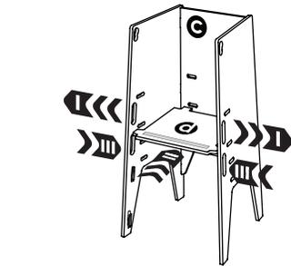
**3** Spread sides apart to insert tabs on Platform (d) into slots on Back (c) at desired height. Push sides together to catch tabs on Platform (d) in slots on sides.
