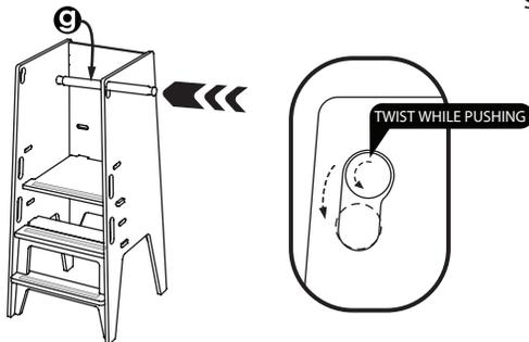
**6** Slide Dowel (g) into hole from side. Twist Dowel (g) while pushing down to lock into place.
