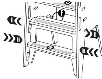
**4** Spread sides just enough to insert Ladder (e). Unless Platform (d) is on lowest setting, also insert Extra Step (f). Push sides together, catching tabs on Ladder (e) and Extra Step (f) in slots on sides.
