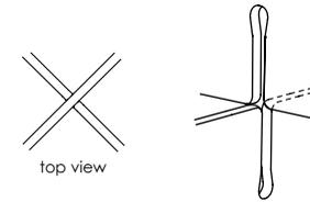
Press the slots to the locked position. This will require some force. **For easiest assembly, position yourself above the joint and use your weight to press down.** There should be no room between the slots when you are done.
