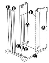
Insert Slats with holes into outer most slots on **Side Panel** (a). Insert remaining **Slats** (a) and **Dowels** (a) into designated places.
