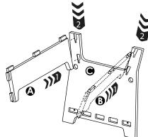
Insert tabs on Braces (A&B) into slots on **Side Panel** press down to lock.
