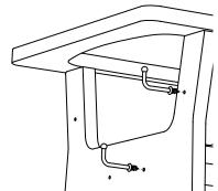
As desired, insert screw-in hooks into holes on outside of Side Panels. If necessary, tighten with pliers with support@sprout-kids.com jaws wrapped with cloth.
