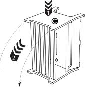
Set second **Side Panel** into position. It helps to start at one side fitting the dowels into the holes and work your way across one at a time. Carefully set upright.
