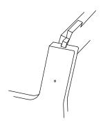
**Grooves on Support Panels** should be oriented inwards as pictured above.
