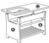
Align up slots on **Table Top** with tabs on **Braces (3)**. Push down until flush with top of Side Panels.
