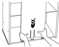
Insert center tab of Partial Back into center slot on Side. Holding the piece as shown, flex the back and push the dovetail tabs into the open slots.
