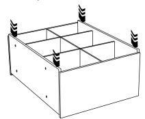
Carefully tip shelving unit onto its back on a hard floor and press down on ends of Bottom and Top Shelves until flush with sides.
