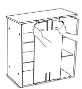
Insert center tab on Back into slot on side. Flexing the Back, push tabs into open slots. Then insert tabs on Top into slots on side.
