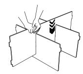
Slide Horizonal Divider into slots on Vertical Dividers, as shown. Set aside.
