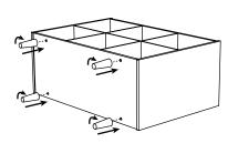
Lastly, screw in the four legs into the Bottom Shelf until tight, as shown.
