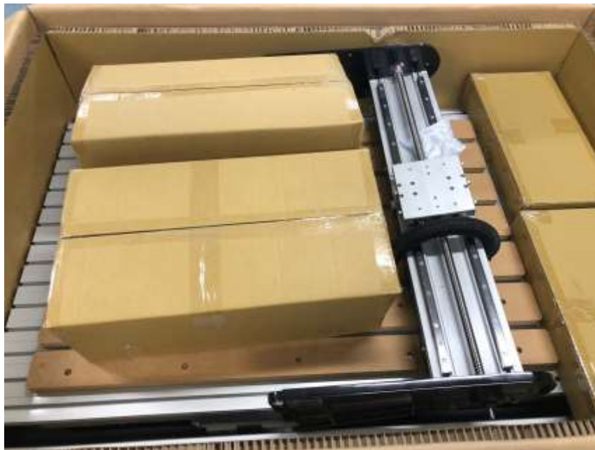
Figure 1: i2R CNC 4 with box cover removed and ready for lifting
