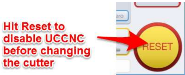
Figure 12: Reset to disable spindle relay
