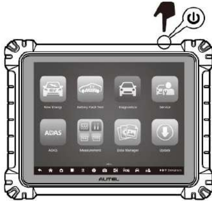
Figure 5-3 Power up the Tablet
