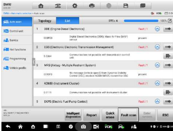
Figure 7-3 Fault Scan on List Screen
