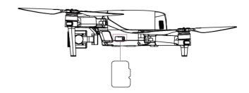
Without Micro SD card, it is also allowed to take photo or record video but the image will be directly stored in the mobile device.
