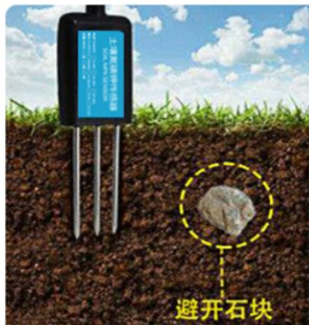
Choose the proper measuring position. Split the surface soil according to the measured deep.
