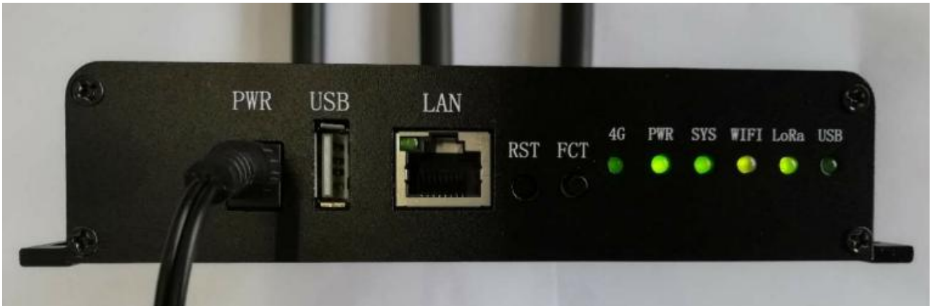
Figure 2- 14 Led instructions in AP/STA mode when connected to cloud server
