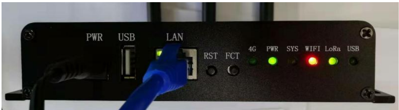
Figure 4-5 Led instructions in default AP mode when connected to cloud server
