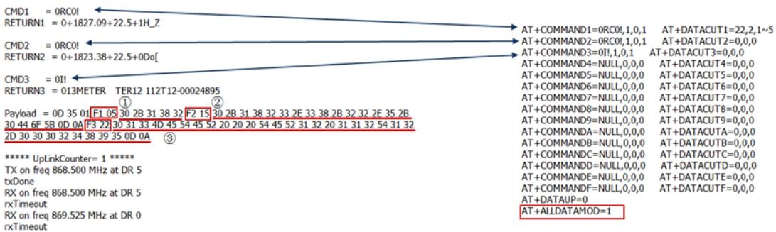
If AT+ALLDATAMOD=1, **FX,X** will be added in the payload, FX specify which command is used and X specify the length of return. for example in above screen, F1 05 means the return is from AT+COMMAND1 and the return is 5 bytes.
