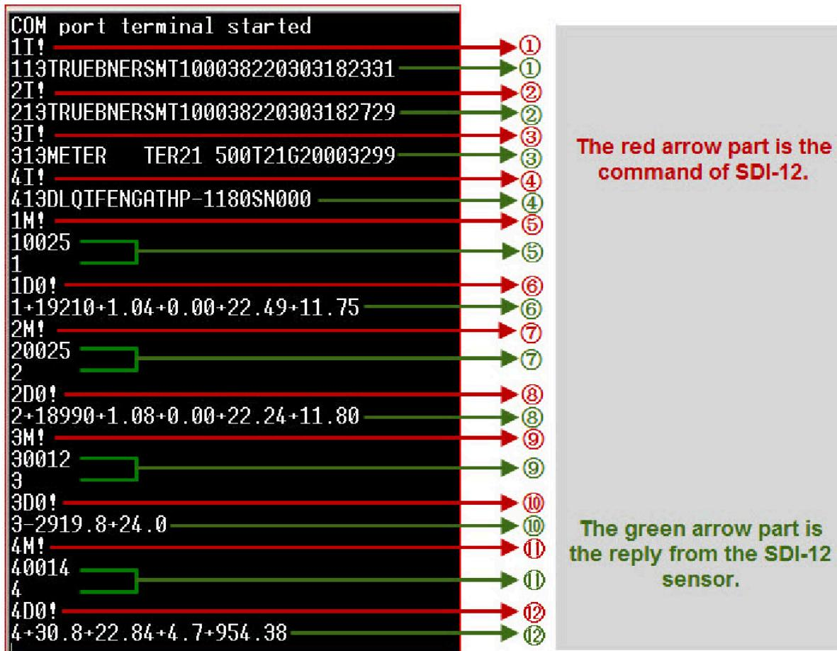
1) The AT+COMMANDx command is applied to the red arrow part, and sends the SDI12 command to the SDI12 sensor:
