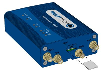
3. To remove the SIM, push the edge of the card in. When released, the card pops out of the device.
