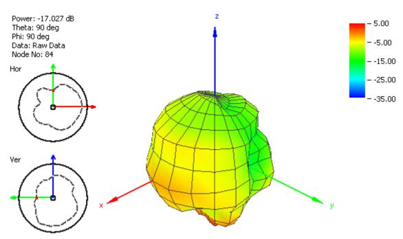
Figure 7. Radiation pattern at 930 MHz on a Piece of Road.
