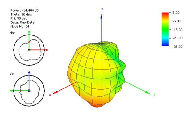
Figure 10. Radiation pattern at 930 MHz in Free Space.
