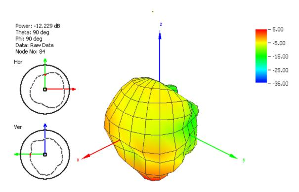
Figure 8. Radiation pattern at 900 MHz in Free Space.
