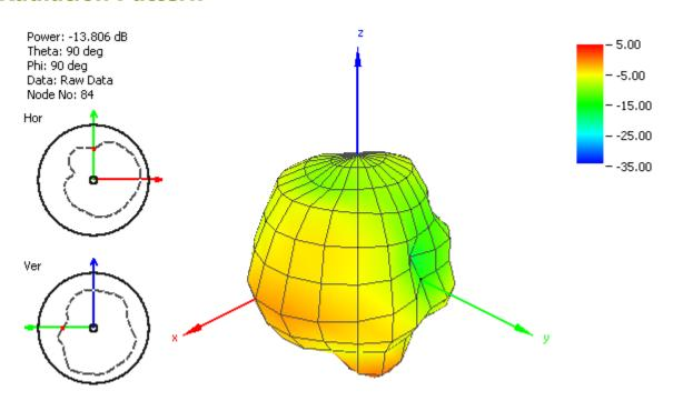
Figure 5. Road Marker ISM Antenna radiation pattern at 900 MHz on Piece of Road.
