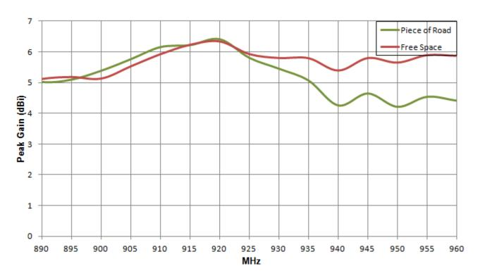
Figure 4. Peak Gain 915MHz Road Marker in Free Space and on Piece of Road
