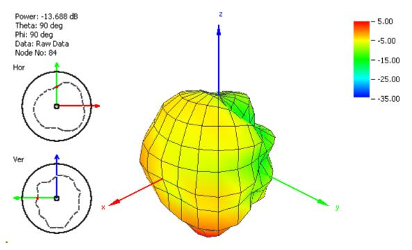
Figure 9. Radiation pattern at 915 MHz in Free Space.
