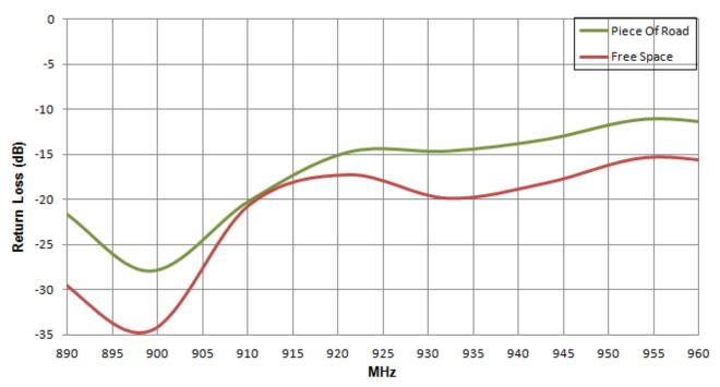
Figure 2. Return Loss 915MHz Road Marker in Free Space and on Piece of Road.
