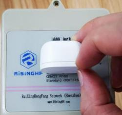
Picture above shows the position of Hall sensor, Place a Magnet close to this position for around 1 second (less than 10 seconds) and release (take away), RHF1S052 will trigger a field test.
