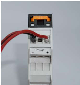
Fig.4 Power supply terminal
