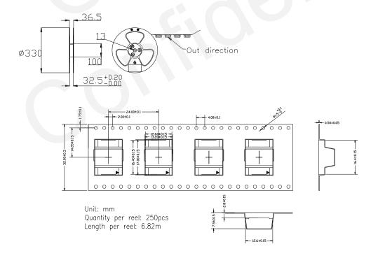
Figure 23: Tape and Reel Specification
