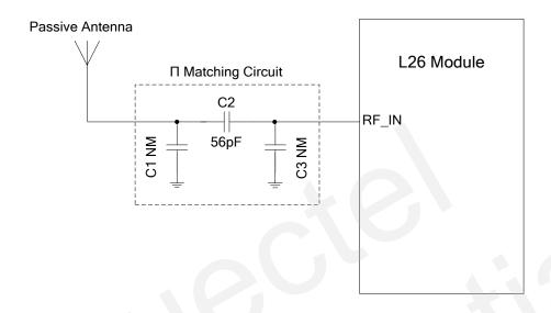
Figure 13: Reference Design with Passive Antenna
