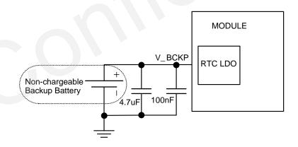
Figure 5: RTC Supply from Non-chargeable Battery
