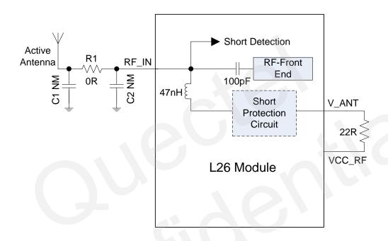
Figure 14: Active Antenna Reference Design with Short Protection
