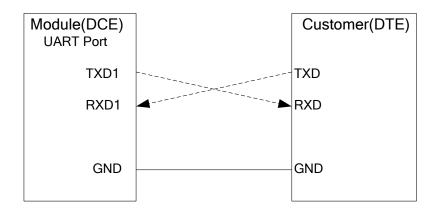
Figure 11: Connection of Serial Interfaces
