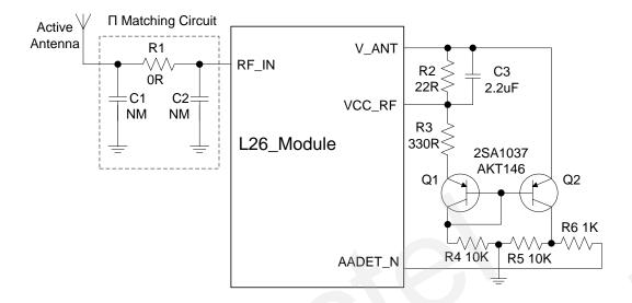
Figure 15: Active Antenna Reference Design with Antenna Detection
