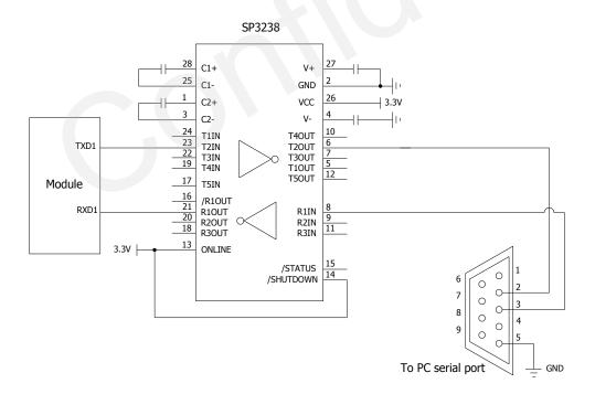
Figure 12: RS-232 Level Shift Circuit
