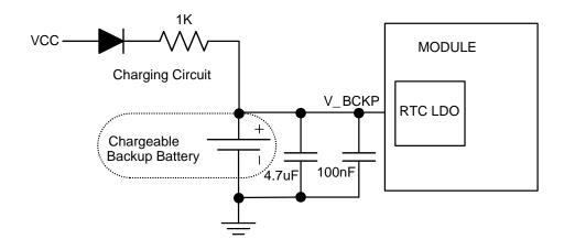
Figure 6: Reference Charging Circuit for Chargeable Battery
