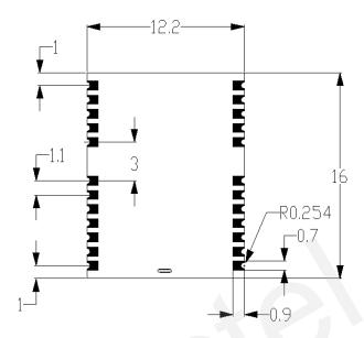
Figure 18: Bottom Dimension (Unit: mm)
