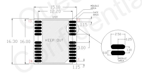
Figure 19: Footprint of Recommendation (Unit: mm)
