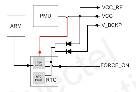
Figure 3: Internal Power Construction
