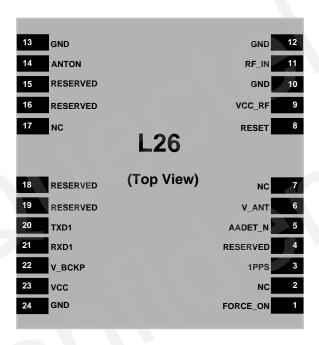
Figure 2: Pin Assignment
