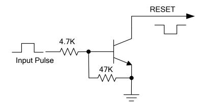
Figure 9: Reference Reset Circuit Using OC Circuit
