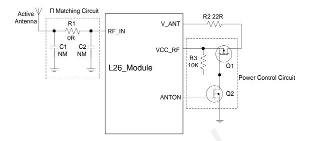
Figure 16: Reference Design for Active Antenna with ANTON
