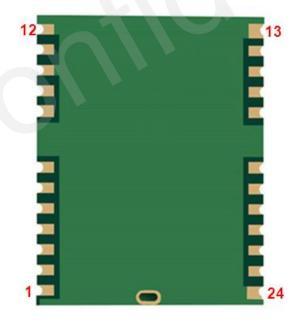
Figure 21: Bottom View of the Module
