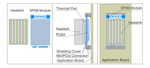
Figure 16: Referenced Heatsink Design
