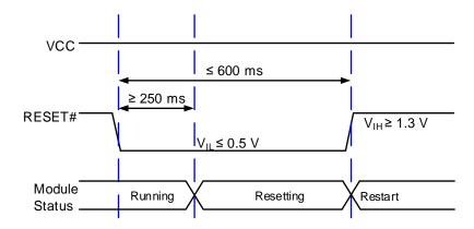
Figure 10: Timing of Resetting Module
