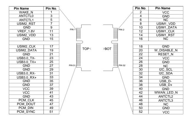
Figure 2: Pin Assignment of EP06 Series
