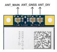
Figure 12: Antenna Connectors on the Module
