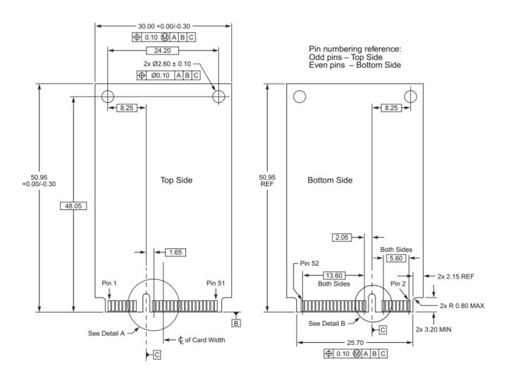
Figure 19: Standard Dimensions of Mini PCI Express
