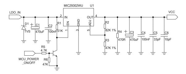
Figure 3: Reference Design of Power Supply
