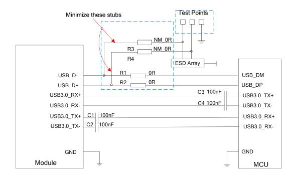
Figure 5: Reference Circuit of USB 2.0 & 3.0 Interfaces
