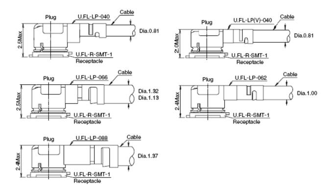
Figure 15: Space Factor of Mating Plugs (Unit: mm)
