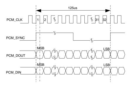
Figure 7: Auxiliary Mode Timing
