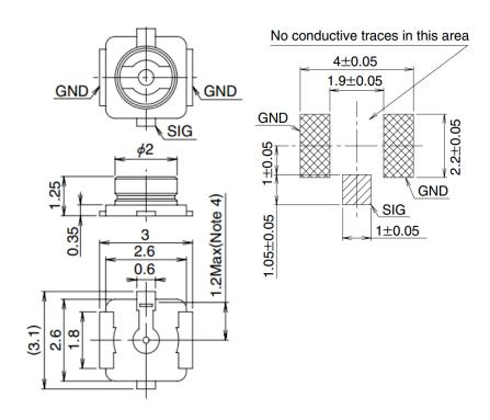
Figure 13: Dimensions of the Antenna Connectors (Unit: mm)
