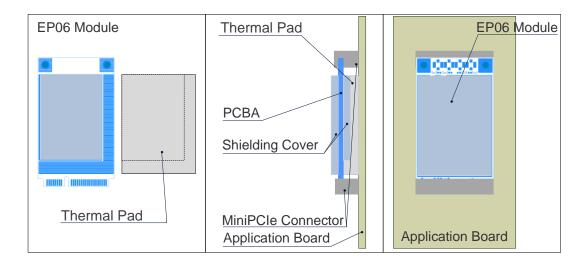
Figure 17: Referenced Thermal Pad Design
