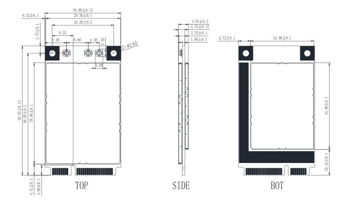
Figure 18: Mechanical Dimensions of EP06 Series
