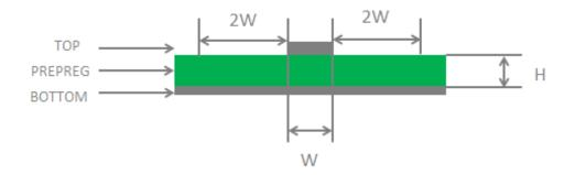
Figure 17: Microstrip Design on a 2-layer PCB
