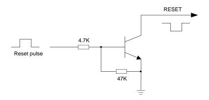
Figure 7: Reference Circuit of RESET with Driver Circuits
