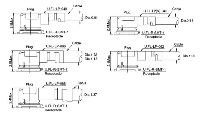
Figure 23: Space Factor of Mated Connector (Unit: mm)
