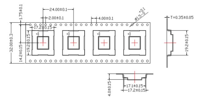
Figure 30: Tape Dimensions (Unit)
