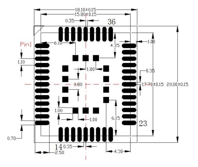
Figure 26: Recommended Footprint (Top View)
