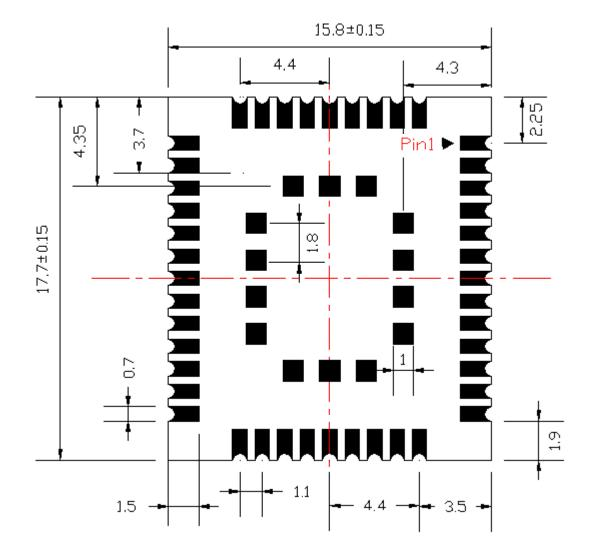
Figure 25: Bottom Dimensions (Bottom View)
