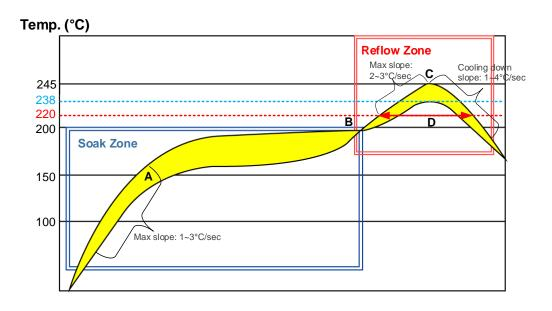
Figure 29: Reflow Soldering Thermal Profile
