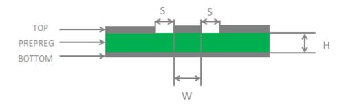
Figure 18: Coplanar Waveguide Design on a 2-layer PCB
