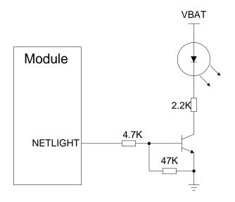
Figure 15: Reference Design for NETLIGHT
