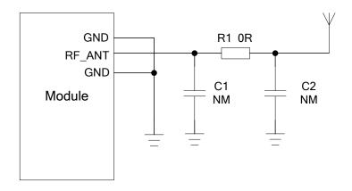
Figure 16: Reference Design of RF Antenna
