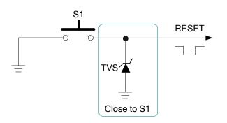
Figure 8: Reference Circuit of RESET with Buttons
