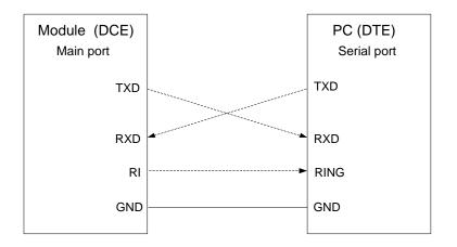
Figure 9: Reference Design for Main Port
