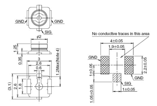
Figure 21: Dimensions of the U.FL-R-SMT Connector (Unit: mm)
