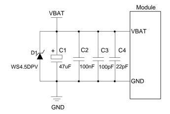
Figure 4: Reference Circuit for Power Supply
