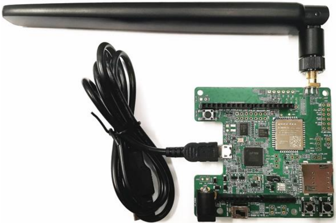
Figure 16: BC660K-GL-TE-B Kit Assembly
