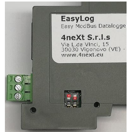
Fig. 6 DIP-SWITCH position for DHCP
