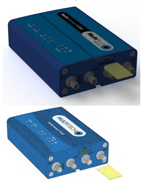
3. To remove the SIM, push the edge of the card in. When released, the card pops out of the device.
