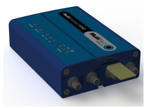
3. To remove the SIM, push the edge of the card in. When released, the card pops out of the device.
