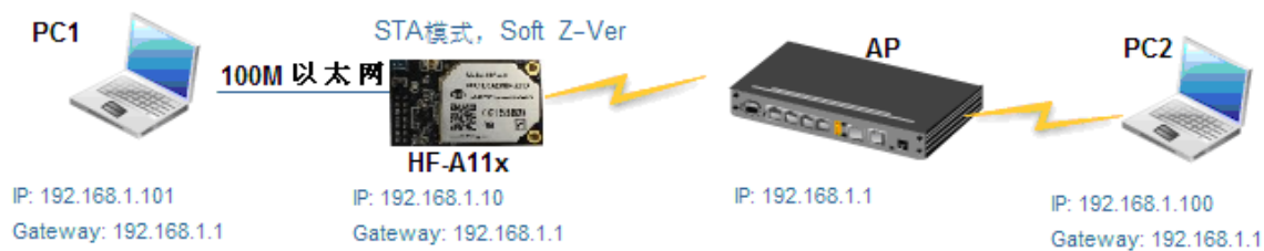
Figure 20. HF-A11 Ethernet Interface Networking (As STA, Z-Ver)
