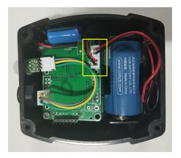
Figure 5.1 Connect battery and capacitor
