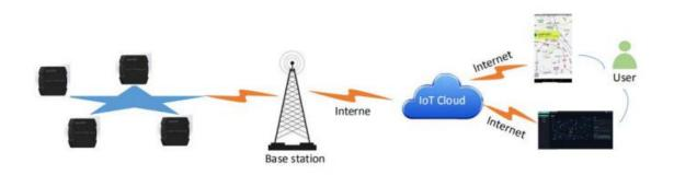
Through the built-in NB-IoT wireless module, it transmits data to the base station through the NB-IoT network, Then transmits the data to the web server and application server through the internet . Finally, the user can monitor the number of
