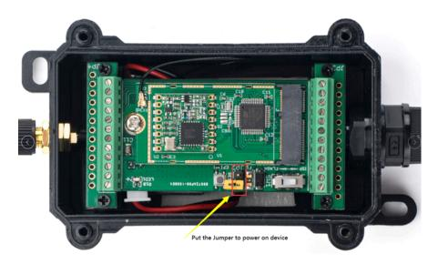
Put the jumper to power on CPL01 and it will auto-join to the TTN V3 network. After join success, it will start to upload sensor data to TTN V3 and the user can see it in the panel.
