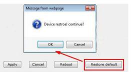
If choose **OK**. The ATC-1200 will be automatic to restart within 15 seconds. We also offer another hardware button to Restore ATC-1200. To find restore button as following photo.
