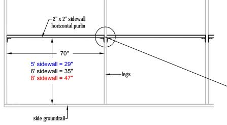
Depending on sidewall height ordered, measuring up from the top of the groundrail place purlin at <u>29" for 5'-0" sides</u> or <u>47" for 8'-0" sides</u>.
