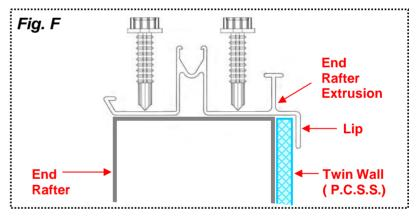
Working your way down, conform the extrusion to the shape of the rafter, while inserting two tek-screws 12 to 16 inches apart down the full length of the rafter. (See photo #3)
