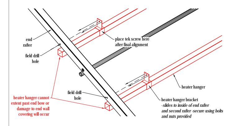
Attach the heater hangers to the end rafter (preferably to the front end rafter) and the second rafter. Be sure that the heater hanger does not extend past the end rafter because it will damage the end wall covering when it is installed.
