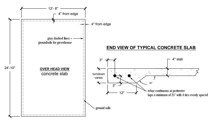
When pouring concrete slab be sure to make the slab 10" longer and 8" wider than your order size. An example is shown above: OVERHEAD VIEW concrete slab shows a greenhouse order for a 12' x 24' Scholar. The slab is poured 12'-8"wide and 24'-10" long. Set front/rear groundrails 4" inward from edge of concrete and side groundrails are set 4" inward from edge of concrete.
