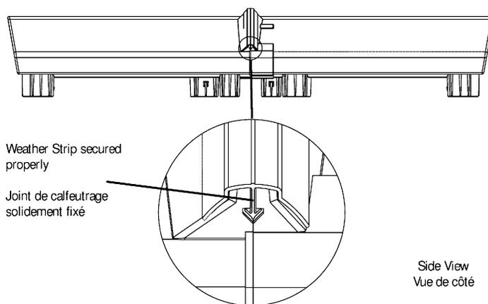
13. With at least 2 people, lift the assembled roof over the Shed and lower into place. **Do not snap into place until all posts are lined up and partially engaged.** Make sure tabs on back panels are engaged before snapping into place (See detail view). Start at one corner and work your way around the shed pressing down at edges of Roof to fully snap connectors in place.
