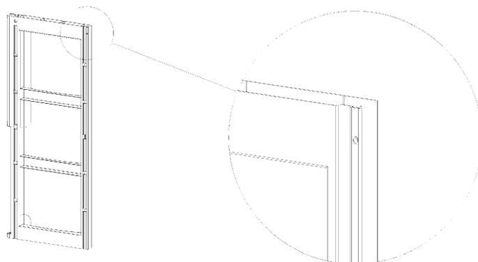
17. Locate door handle assembly receptacle on the Right Door O. Insert Right Door Handle H into door handle receptacle at an angle.
