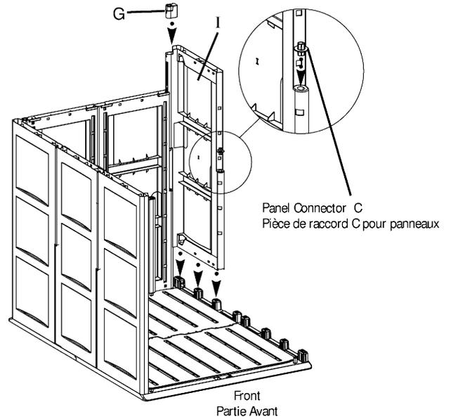
8. Insert remaining Panel Connector C into remaining Panel B. Press down into place.
