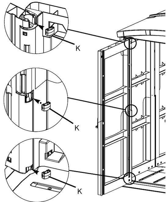
23. With Left Door open, line Right Door O up in closed position, and slide to right onto the hinges.
