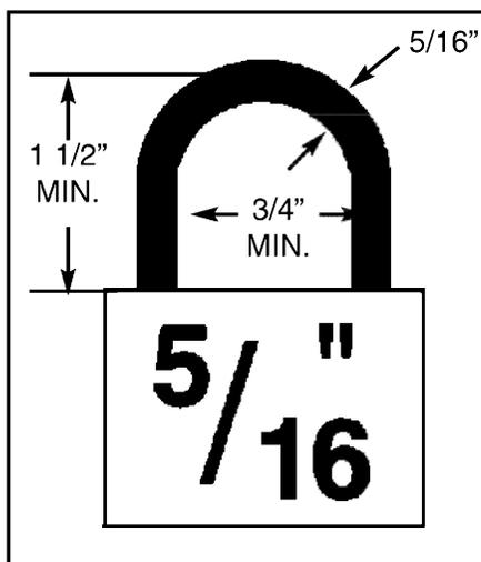
To properly lock your shed using the Padlock Assembly feature, 5/16" padlock is recommended.
