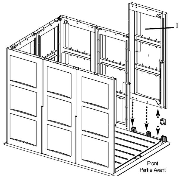
10. Insert Front Cap Plug E into Floor Panel. Press until part snaps in place. If necessary, use foot to press into place.
