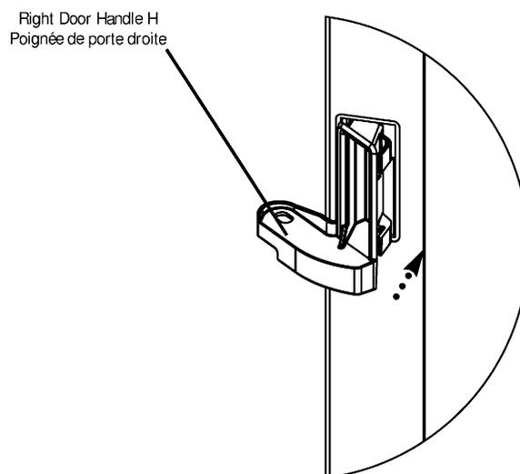
18. Locate door latch assembly housing receptacles in the lower left and upper left corners of the Right Door. To insert Door Latch Housings into door latch receptacles **first position Door Latch Assembly Housing Tabs so they point towards the edge of the door**. Place the Tabs behind the front wall of the door and press until part snaps in place.
