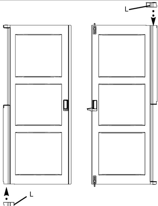
21. Line Left Door X up in closed position and slide to left onto the hinges.
