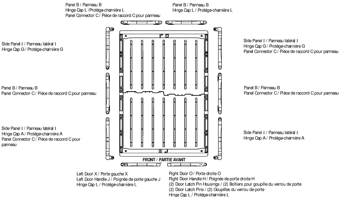
Top view of shed (without roof) showing where panels are used.
