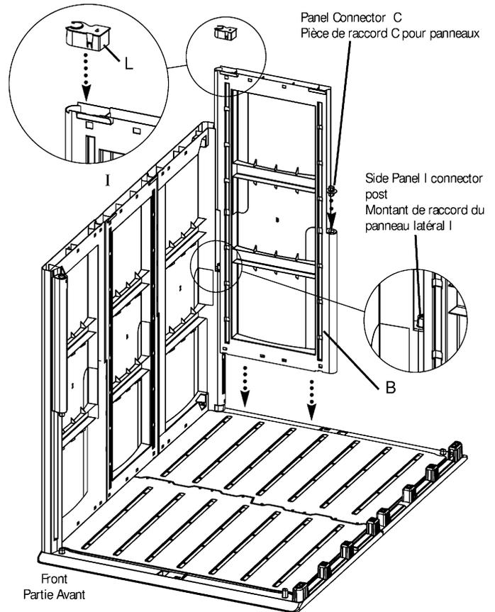
6. Insert Back Floor Post D into Floor. Press until part snaps in place.
