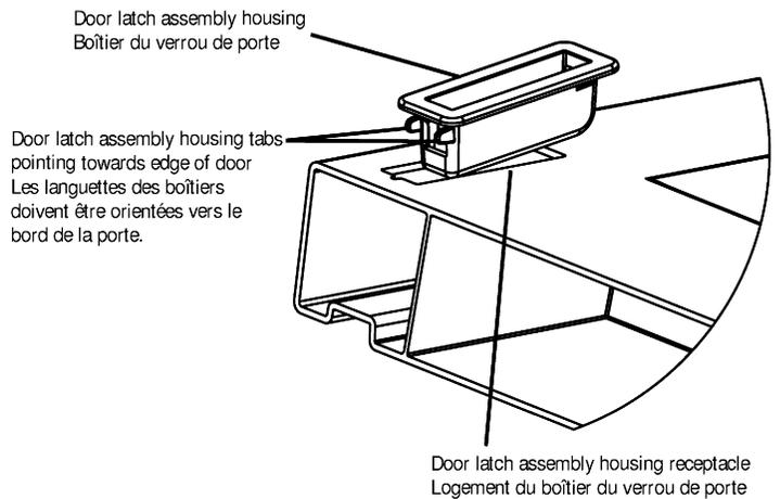
19. Starting with the **BOTTOM** Door Latch insert the square end of the Door Latch Pin **UP** into the Door Latch Housing. Once square end of Pin is inserted. Push Door Latch Pin **downward** to engage snaps that secure it inside housing.
