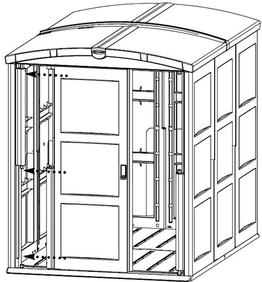
22. Open the Left Door fully and stand inside shed facing the door hinges. Insert the three Hinge Retainers K. Press into place or tap in with a small mallet or hammer if needed.
