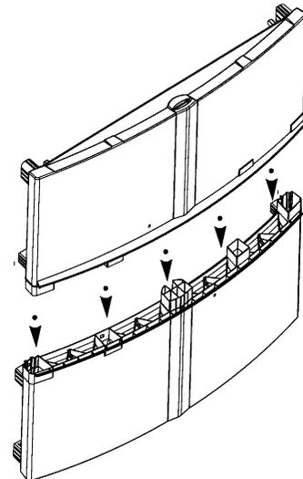
12. Liberally apply the provided lubricant to at least 4 places along the length of the roof seam. This will make it easier to insert the weather strip.
