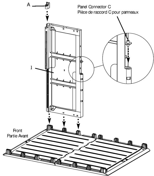
3. Insert one Panel Connector C into one Panel B. Press down into place.
