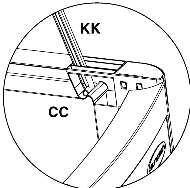
23. To open the Lid to the 6 inch position, lift Lid up past 6 inches, pull Prop Rod towards outside of Upper Side Panel, and lower lid until the stop hook engages with the side panel. This allows front doors to be opened without lifting Lid all of the way.
