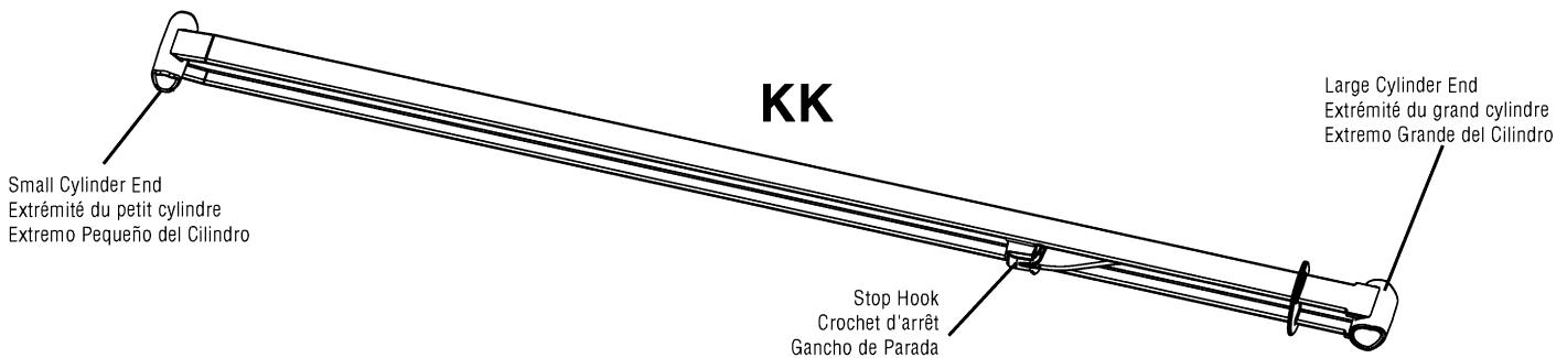
20. Rotate the Lid Support Prop Rod (KK) so that the small cylinder end will pass through slot in the top front of Upper Side Panel (CC or EE as Prop Rod can be placed on either right or left side).
