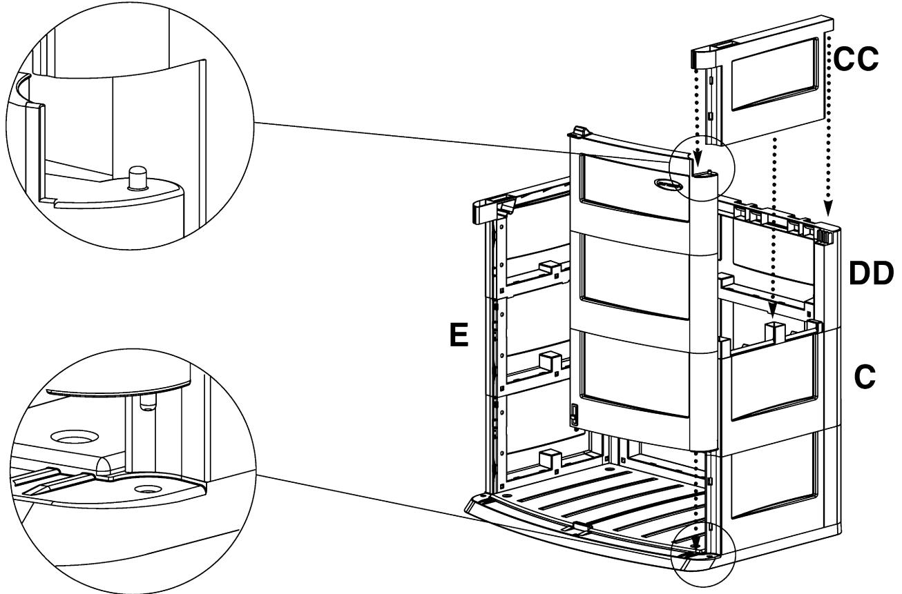
14. Place right door assembly by positioning the door peg (which protrudes from the Lower Door Cap) into the door peg receptacle located in the Base.
