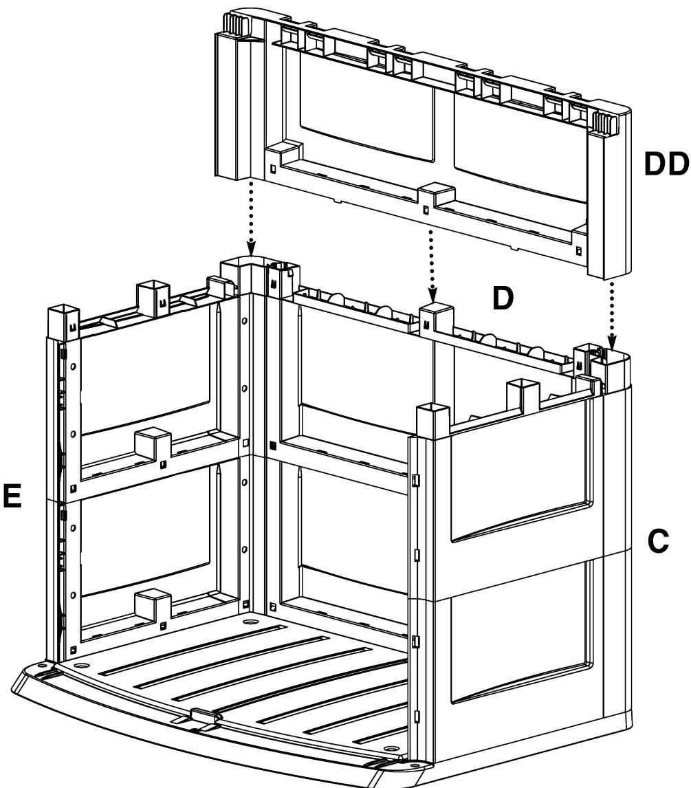
13. Place Upper Back (DD) onto Lower Back (D) making sure to connect to Lower Sides (E,C). Press down until Upper Back snaps into place.
