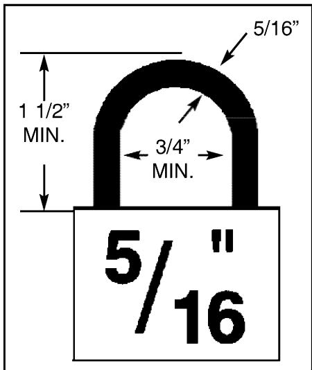
**Securing Your Shed:** To properly lock your shed using the Padlock Assembly feature, 5/16" padlock is recommended.
