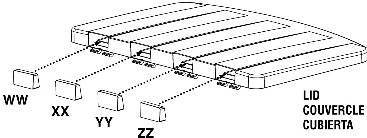
18. Assemble Lid by taking Lid End Caps (WW, XX, YY, ZZ) and pushing them into the respectively marked openings in the Lid.
